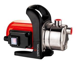
Stainless steel garden jet pump with 800W power. It has a maximum flow rate of 3000L/h, with an immersion depth of 8m and a maximum manometric height of 40m. It has a 10m electric cable, the maximum temperature of the fluids is 35°C. With a power supply voltage of 230 V 50 Hz, it has an IPX4
