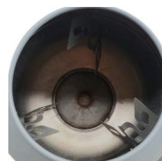
"V" shape mixing blades
